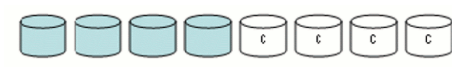
Gambar 20.5. (b) RAID 1: mirrored disk
