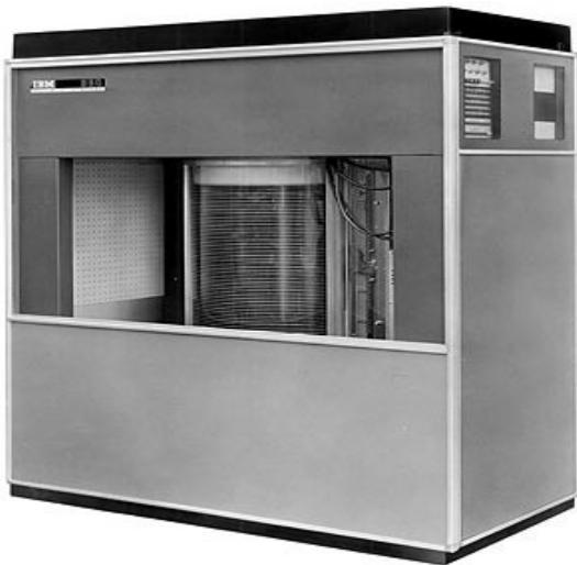
The IBM 350 disk storage unit model 1 (151 cm x 171 cm x 50.2 cm) was announced on September 4, 1956. IBM 350 had 100 surfaces @ 100 tracks. Each track had 5 sectors @ 600 bits. The disk spun at 1200 RPM. The seek time was about  $(10 + 10 \text{ Tr}) \text{ mS}$  where "Tr" was the Track differences. Switching time between surfaces was assumed 0 mS. At that time, the main purpose of IBM 350 was to store "6 bits" characters.
